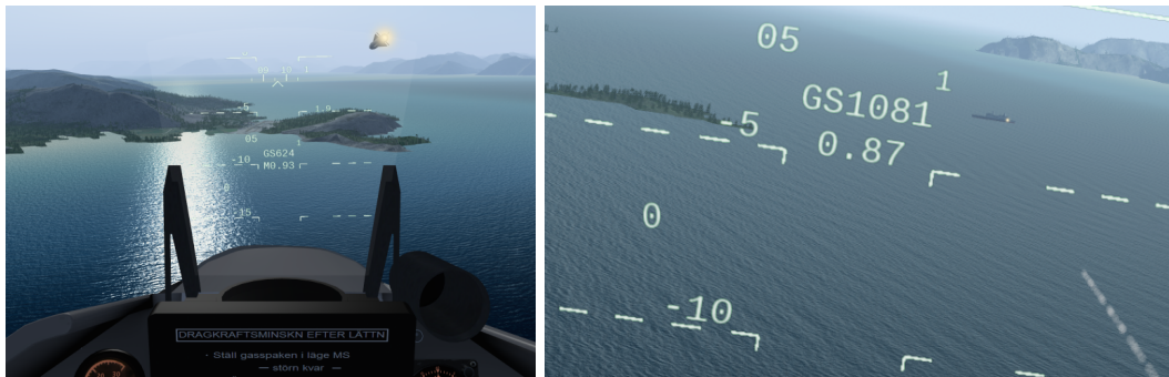
Figure 7.2: Rb 05A flare for visual guidance. On the left, the missile is entering the pilot's field of view just after launch. On the right, the missile is about to hit the target ship, and the missile flare is visible over the ship
